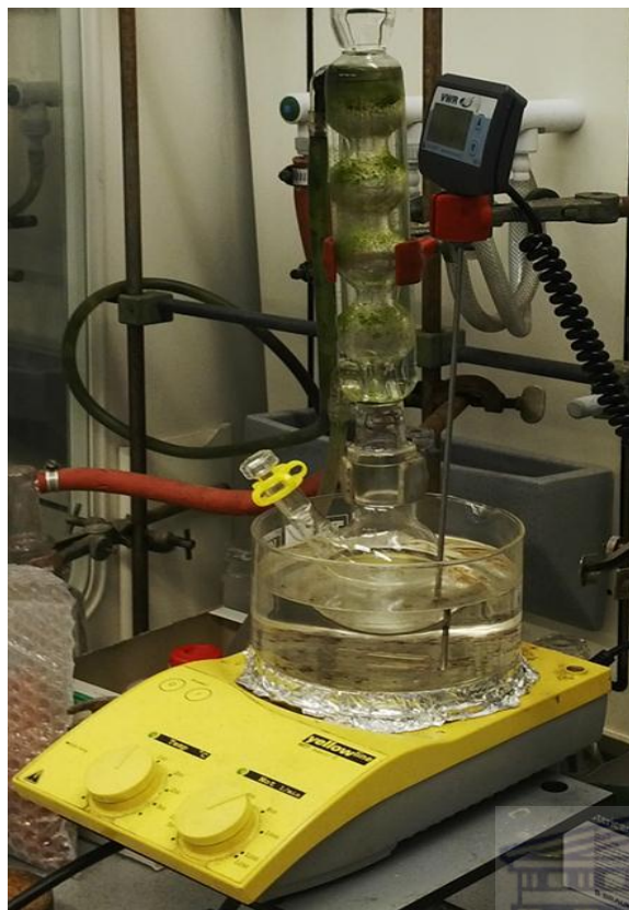
Figure 3.5: Set up for the synthesis of the precursor 1-phenyl-2-ethylpropanone.
