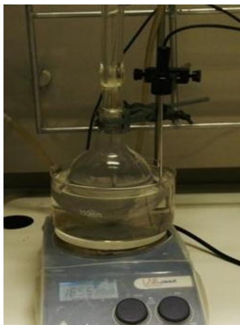
Figure 3.3: Set up of the acid leaching of coal fly ash.
