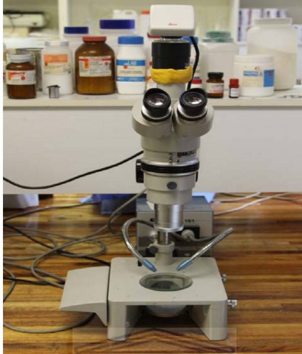
Figure 3.11b: Stereomicroscope (Nikon SMZ 10) and digital camera (Leica DFC 290)
