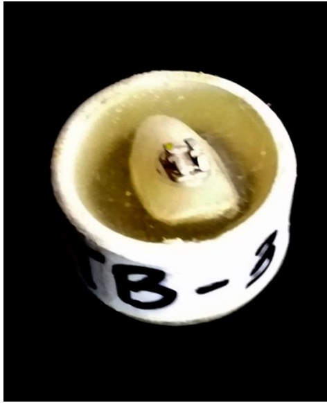
Figure: 7. Crown embedded and bonded with a metal bracket. Labelled according to particular groups
