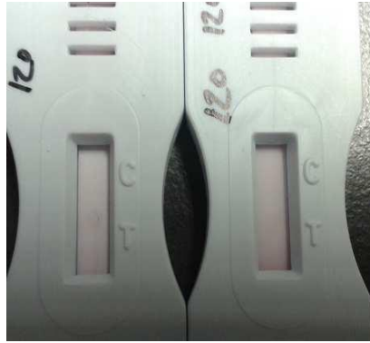
Figure 3.15: Picture showing tests run with CD4 on the membrane and gp120 on the conjugate. The left test was run using buffer only and the right test was run with gp120 spiked into the buffer at a concentration of 8 \mu\text{g/ml} in triplicate.
