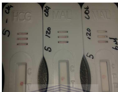
Figure 3.19: Tests run with CD4 on the membrane and Molecule 7 on the conjugate. The left test was run with buffer only. The middle test was run with buffer spiked with gp120 to 8 \mu\text{g/ml} . The right test was run with buffer spiked with gp120 to 18 \mu\text{g/ml} .
