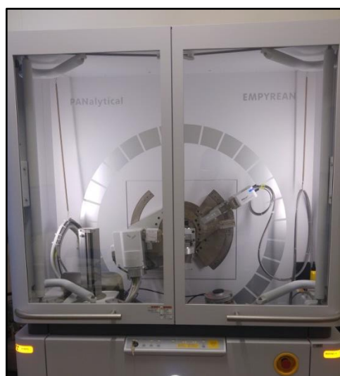
Figure 3.19: Empyrean XRD system (NMISA, Pretoria).
