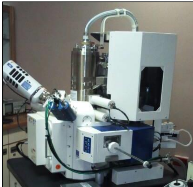
Figure 3.14: Zeiss Auriga FEG-SEM (EMU, UWC, Cape Town).
