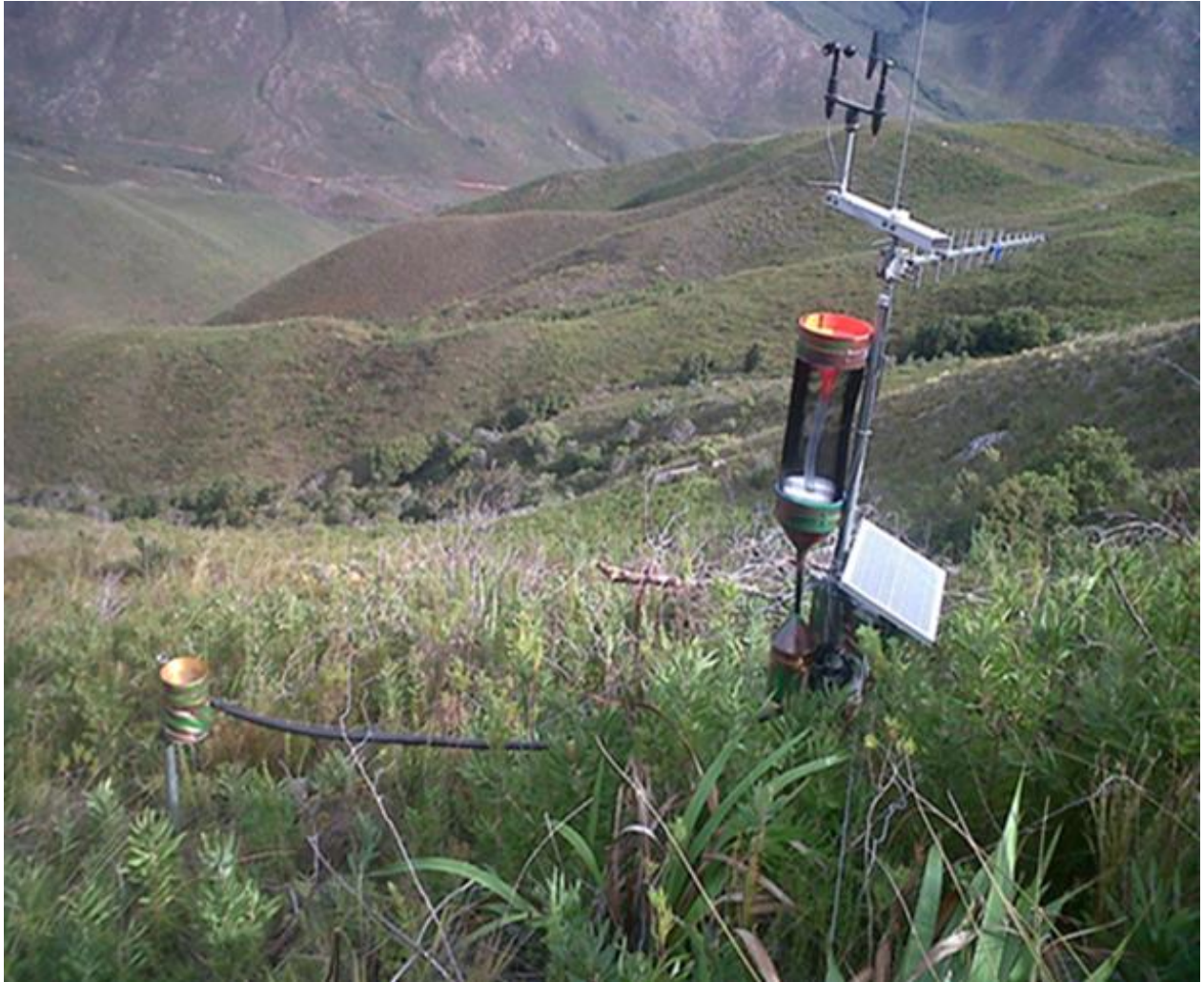
Figure 3.6: Louvred screen fog (Right) mounted on top of a rain gauge with another rain gauge on the left to assess amount of precipitation falling as rain.
