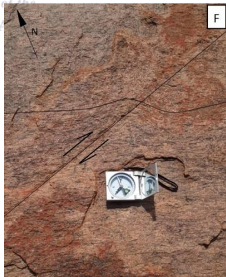
Figure 4-18. a) pi-diagram of 48 joint measurements plotted as points. (b) Rose diagram of the 48 joint measurements displaying a NE/SW strike orientation. (c) Non digitized image of the N/S joints cross cutting the NE/SW joints. (d) Digitized image of the N/S joints cross cutting the NE/SW joints. (e) Non digitized image of dextral shearing along the NE/SW joints (f) digitized image of dextral shearing along the NE/SW joints.
