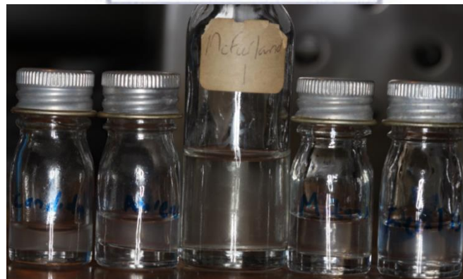
Figure 2: Calibration of suspensions to McFarland 1 turbidity
