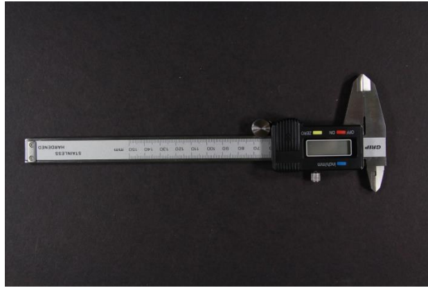
Figure 6: Digital calliper used during the investigation
