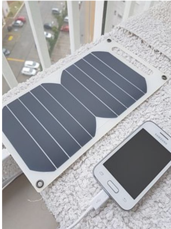
Figure 2. 1: Application of flexible thin film solar panel for charging of mobile phones.
