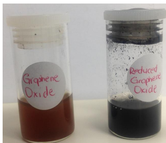
Figure 3.3: Colour comparison of 1.8 mg.ml -1 of graphene oxide (brown) and reduced graphene oxide (black), respectively.
