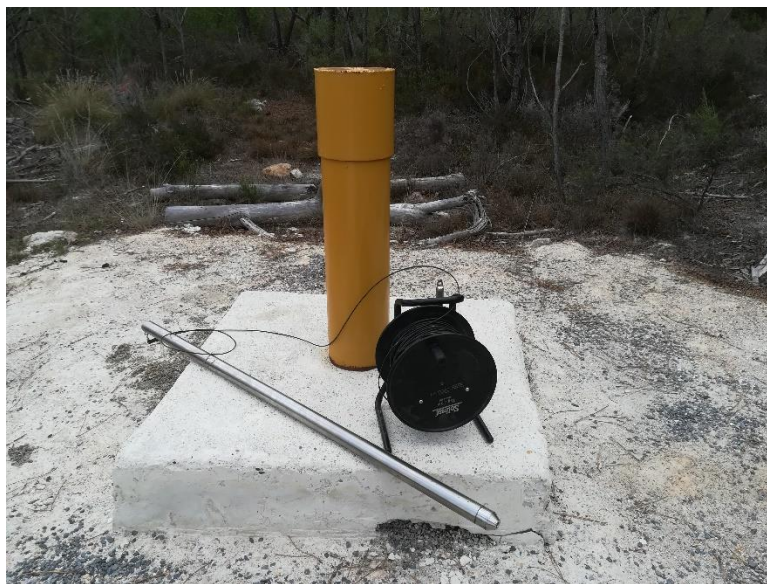
Figure 4.2: A stainless-steel point source bailer with a tagline for collecting groundwater samples
