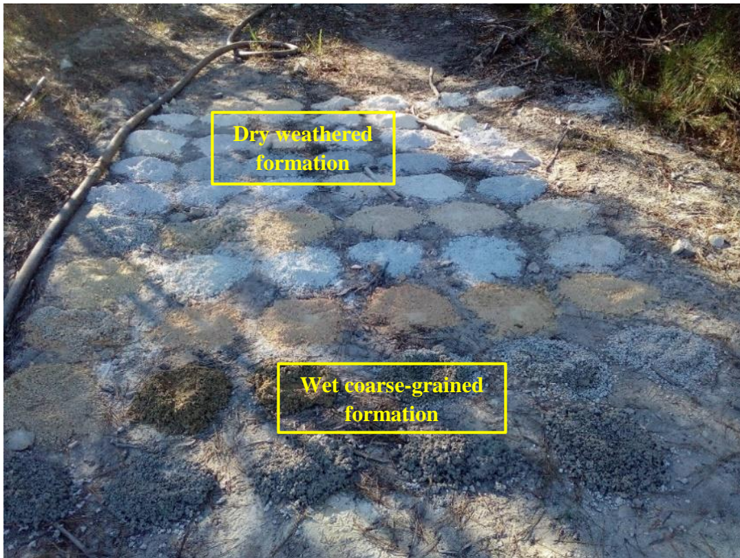
Figure 5.6: Brittle fine-grained sandstone and wet coarse-grained sandstone from BH9
