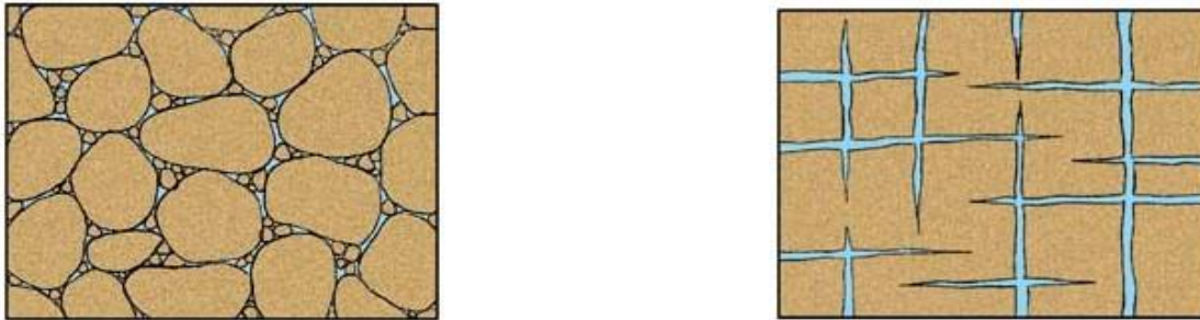
Figure 3.1: Primary porosity (left) and secondary porosity (right) of a rock matrix (Source: https://dpiuwe.tas.gov.au )
