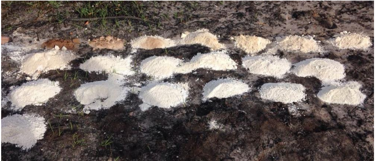
Figure 5.5: Weathered brittle sandstone from BH13
