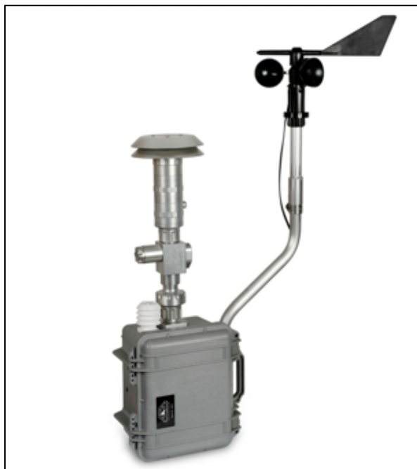
Figure 5-23: ARA N-FRM sampler(ARA, 2016)
