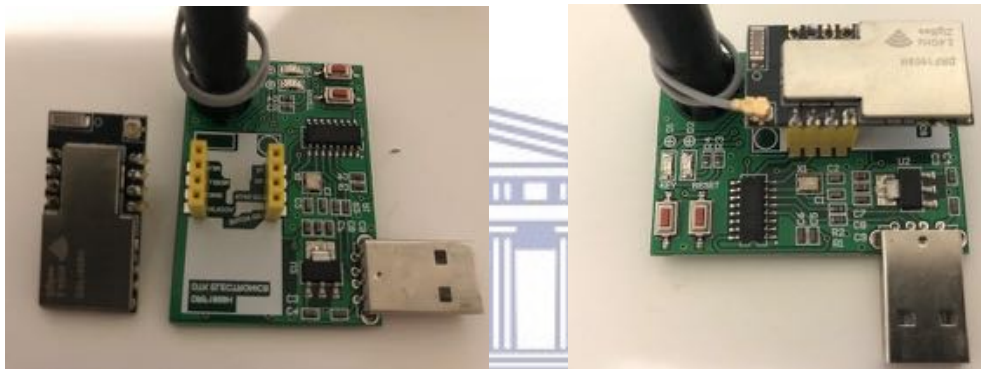
Figure 4-2: Zigbee module wiring instruction diagram
