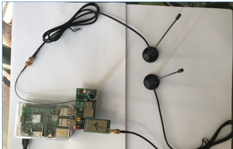
Figure 5-2: Raspberry Pi server placed at the apartment with LoRa and Zigbee modules
