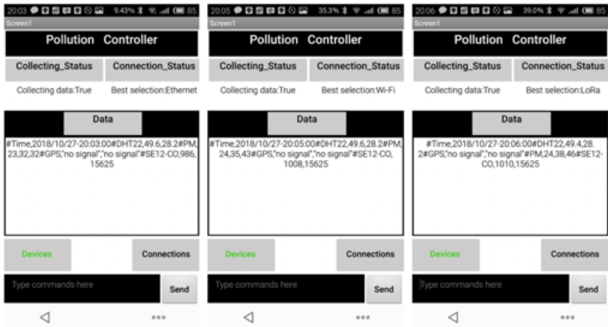
Figure 5-4: Communications of the control app, Ethernet(a), Wi-Fi(b), LoRa(b)
