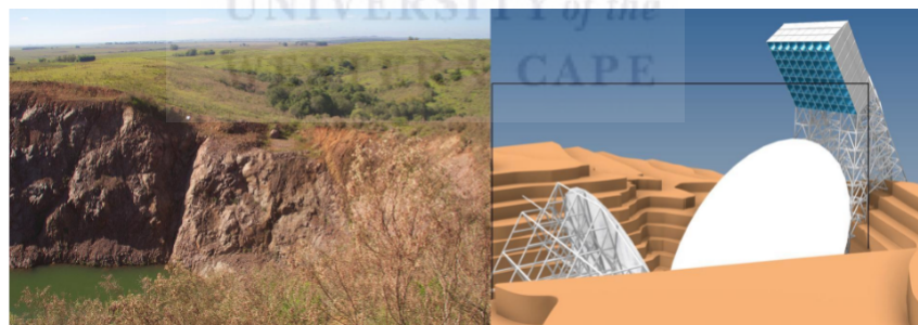
Figure 1.16 On the left is a picture of the Castrillon quarry which is the proposed site of the BINGO telescope. On the right is an engineering drawing of the telescope with primary, secondary and focal plane array of horns in position. The black box in the right hand figure is approximately the plane of the picture on the left. From the paper of of Battye et al. 2016 about the update on the BINGO 21 cm intensity mapping experiment.
