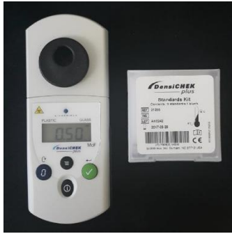
Figure 4- 1: DensiCHEK Plus ® device, used to standardize the density of the inoculum to 0.5 McFarland.
