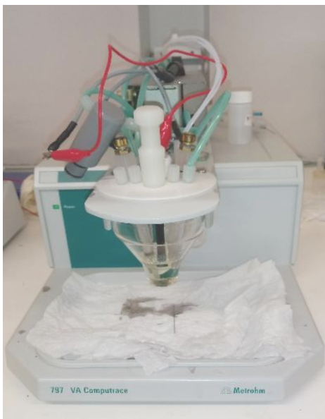
Figure 10: Computrace Potentiostat instrument 797 VA
