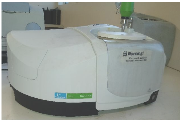
Figure 11: Image of FTIR Spectrometer
