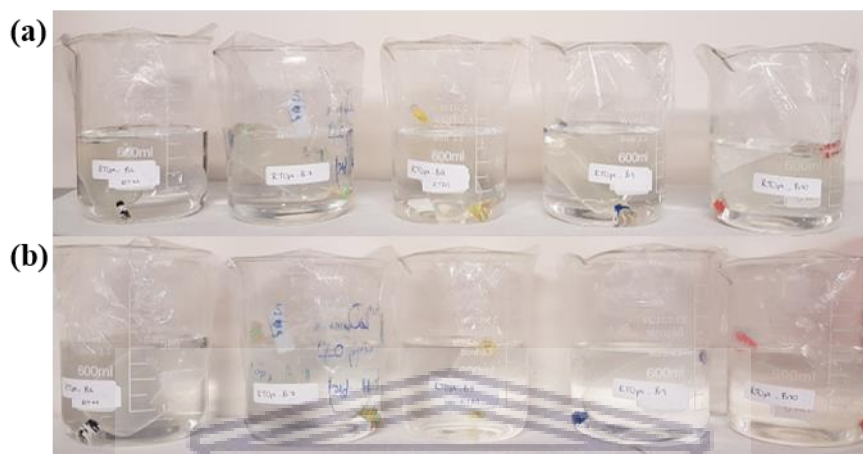
Figure 91. The dialysis of amine-capped carbon dots for the reaction-time optimisation, (a) before, and (b) after dialysis.
