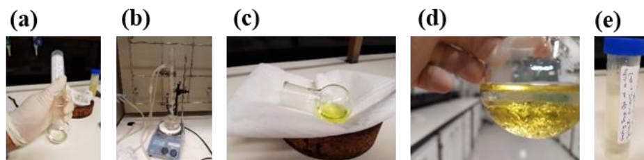
Figure 11. The synthesis of amine-capped carbon dots: (a) transfer of reagent mixture (citric acid (CA) and branched polyethylenimine (BPEI)) into round bottom flask, (b) heating of reagent mixture in a silicone-oil bath with a reflux condenser, (c) cooling of the resultant amine-capped carbon dots (a-CDs) to room temperature, (d) resuspension of the a-CDs in deionised water, and (e) storage of sample.
