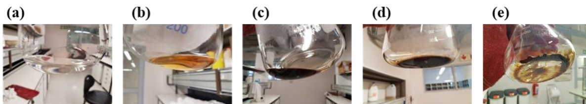
Figure 15. Synthesis power optimisation of plain carbon dots from the lowest to the highest power, namely (a) 90 W (10 %), (b) 270 W (30 %), (c) 450 W (50 %), (d) 720 W (80 %) and (e) 900 W (100 %).
