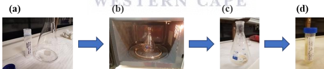
Figure 7. Microwave-assisted method for synthesis of plain carbon dots: (a) mixing of reagent materials in a 250 mL Erlenmeyer (conical) flask, (b) placing of the reagent mixture into the microwave and heating thereof, (c) cooling of product to room temperature, and (d) storage of product after resuspension in DI water.
