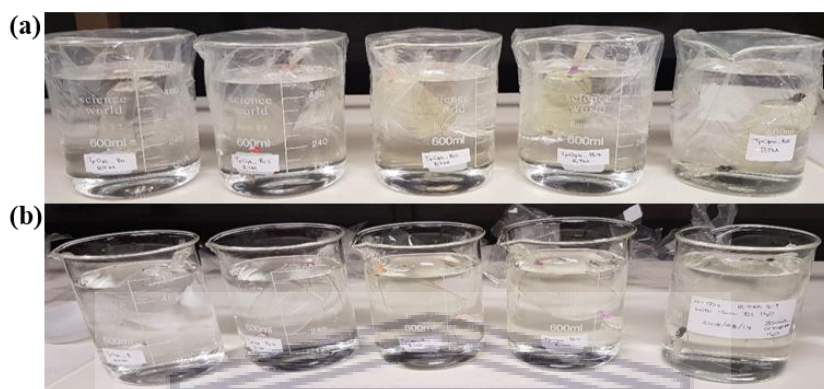
Figure 88. Dialysis of amine-capped carbon dots from the lowest temperature to the highest temperature, (a) before, and (b) after dialysis.
