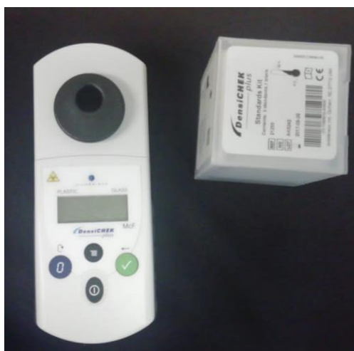
Figure 4-4: DensiChek device used to adjust the inoculum to 0.5 McFarland standard
