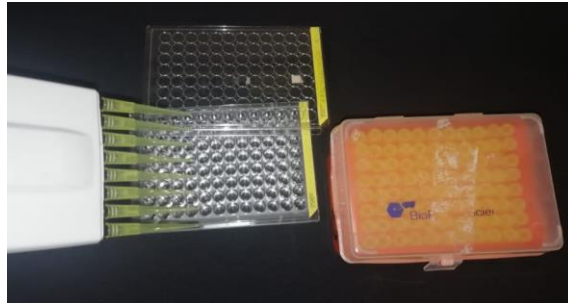
Figure 4-6: 96 well plate used in serial dilution with the multichannel pipette
