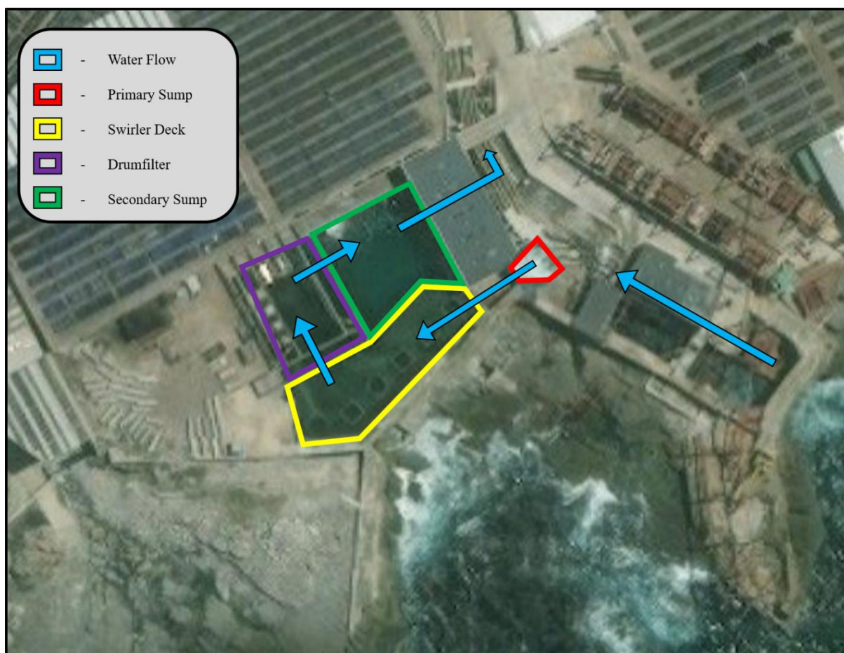
Figure 2.2 A map representing the flow of water through the Primary Sump, drum filter and Secondary Sump at Abagold. Image acquired from Google Maps.
