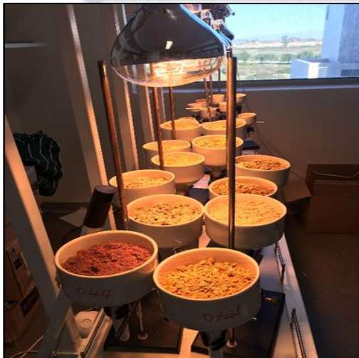
Figure 7.10: Leach column test heat lamp on
