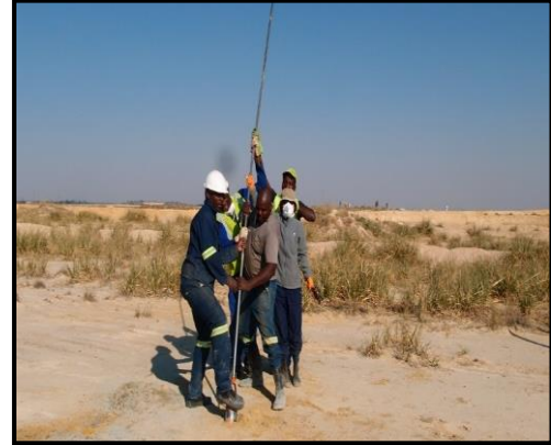
Figure 4.11: Using hand auger to collect samples
