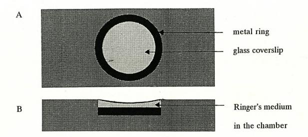
Figure 2: Perspex chambers
