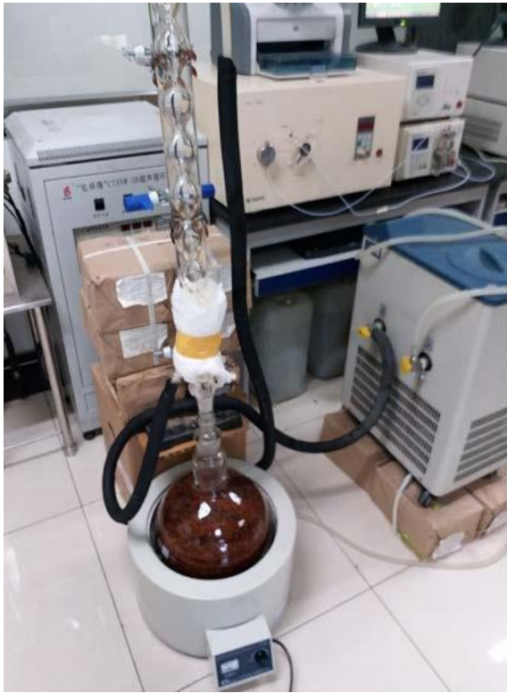
Figure: 2.4: A Soxhlet apparatus that was used for solid-liquid extraction of the medicinal plants, Olea , Rooibos and Centella .
