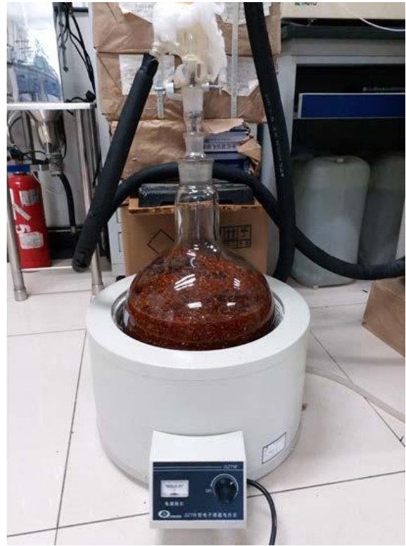
Figure: 2.4: A Soxhlet apparatus that was used for solid-liquid extraction of the medicinal plants, Olea , Rooibos and Centella .
