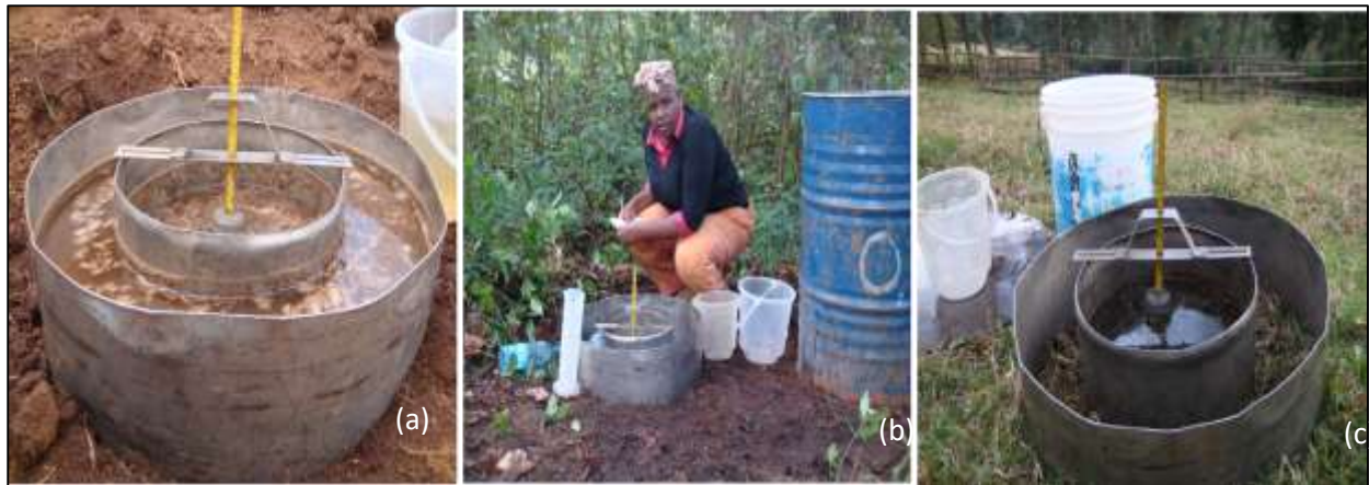
Figure 6.7: Measuring soil infiltration using double ring infiltrometers in (a) cropland (b) forest and (c) grazed lands in the dry season February 2016.
