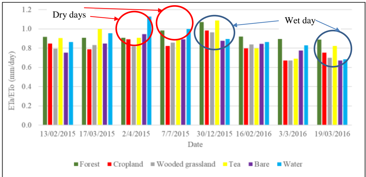
Figure 5.13: Variation of ET_a/ET_o ratio of some selected days in different land use/cover types
