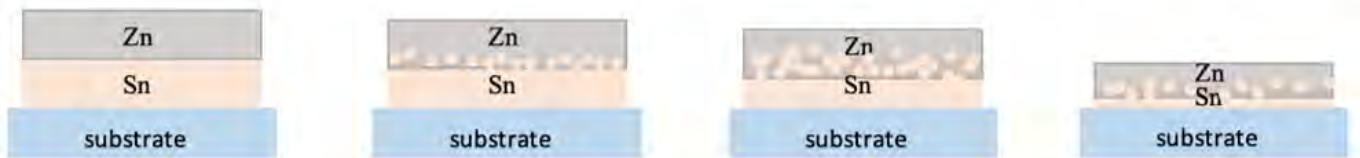
Figure 4.25: Depiction of the Zn and Sn atoms as laser fluence increases.
