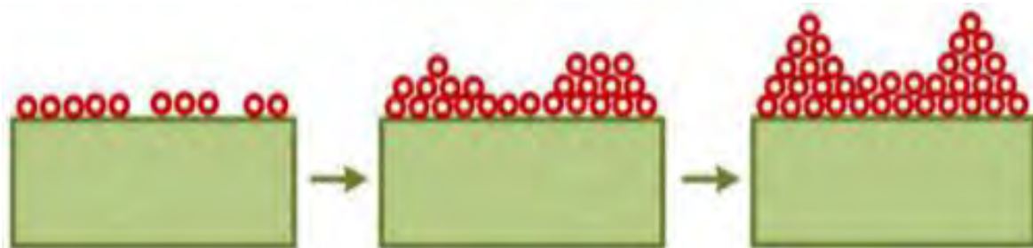
Figure 1.10: Schematic diagram of Stranski-Krastanov growth mode [1.24].
