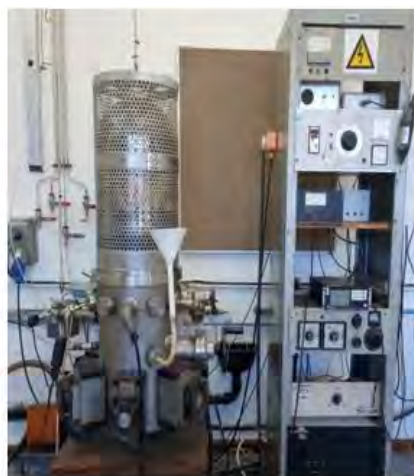
Figure 3.1: Electron beam evaporation system at iThemba LABS that was used for deposition of thin films.
