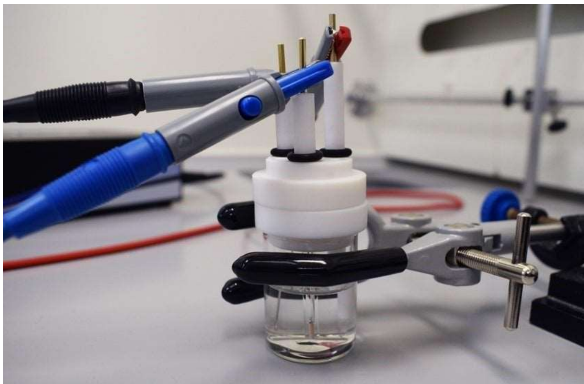
Figure 2.5 Example of a three-electrode system.
