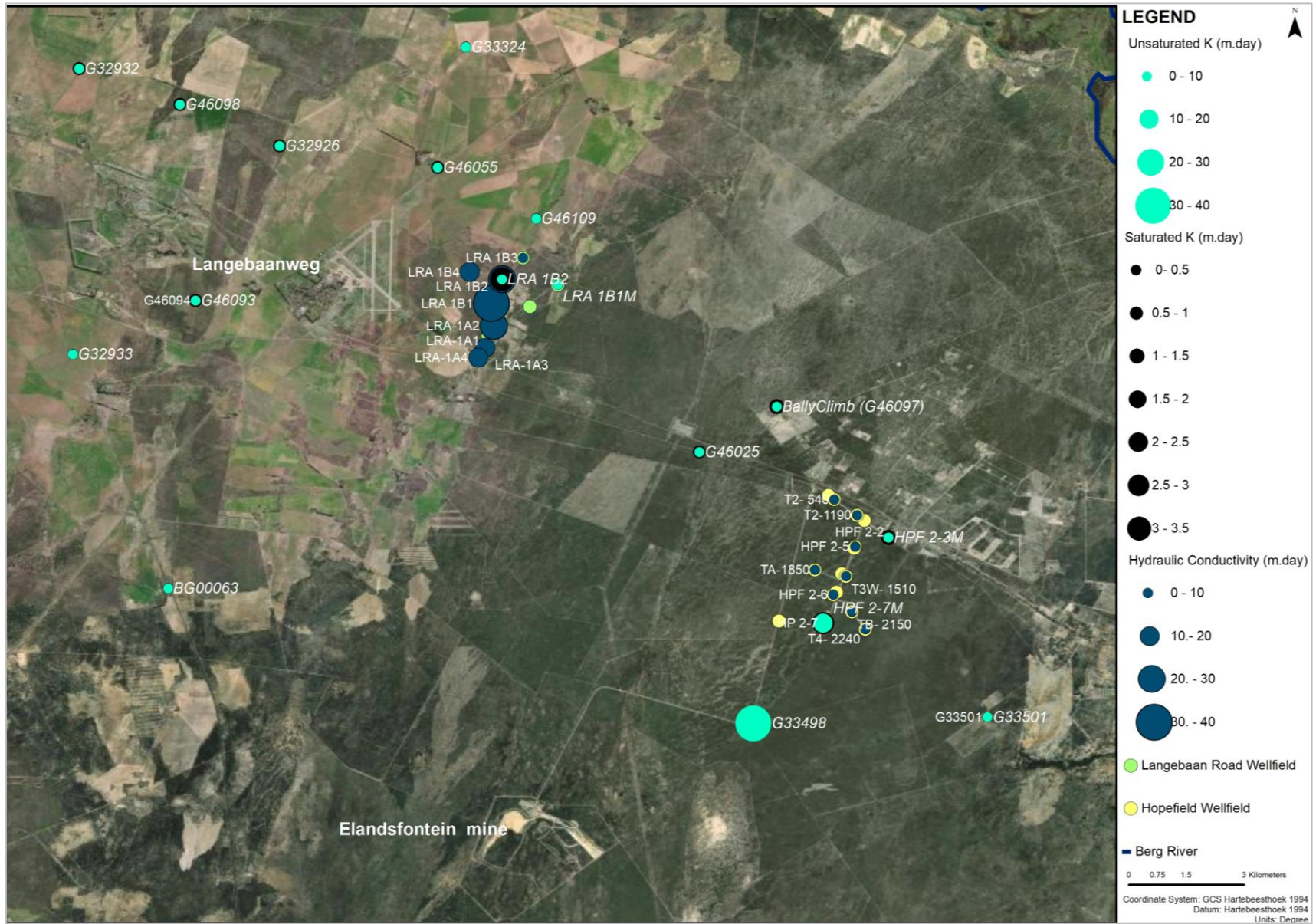
Figure 5-17: Spatial distribution of hydraulic conductivity within the Langebaan Road and Hopefield region identifying aquifer zones best suited for MAR.
