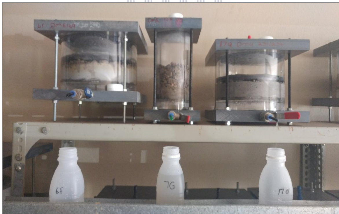
Figure 4-10: Aquatico's static water leaching column setup following the USEPA 1314 percolation column method.
