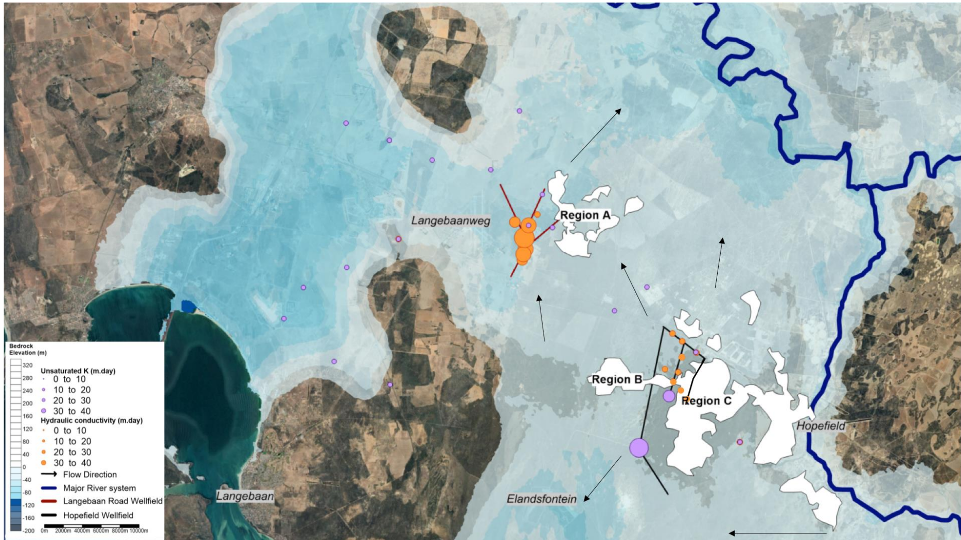
Figure 5-18: Sites identified for Managed Aquifer Recharge within the Saldanha Bay Local Municipality
