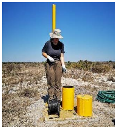
Figure 4-3: D-T-H logging using a YSI attached to a tagline to measure depth specific EC and temperature
