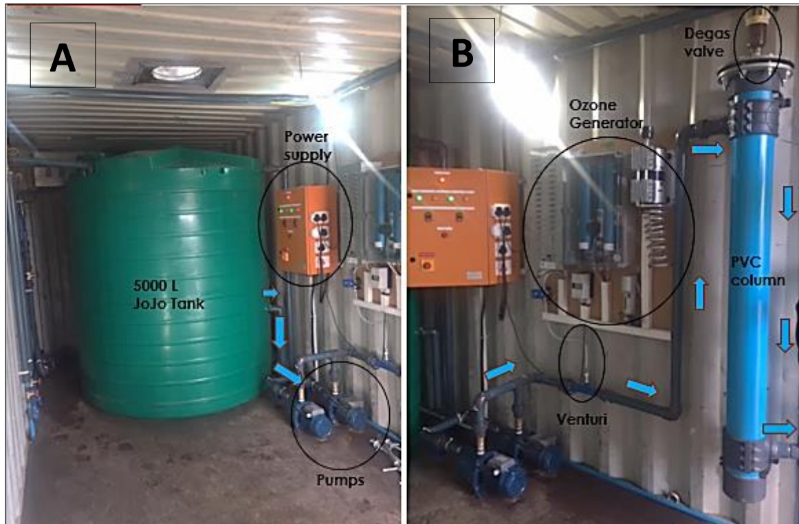
Figure 4.5: The groundwater treatment set-up (using ozonation) inside the shipping container, displaying: A. The 5000 L JoJo tank, power supply, two electrical pumps. The electrical supply was used for both electrical pumps to force water out of the JoJo tank and through venturi's to be dosed with ozone ( O_3 ) B. and O_3 generator, venturi's, degas valve, PVC column and the overall flow direction inside the container.
