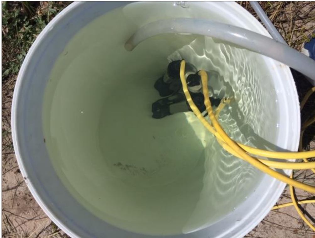
Figure 4.10: Submerged electrical conductivity (EC), pH, temperature, and dissolved oxygen (DO) probes in a 25 L bucket, used to collect field measurements at monitoring boreholes at the study site, Atlantis.
