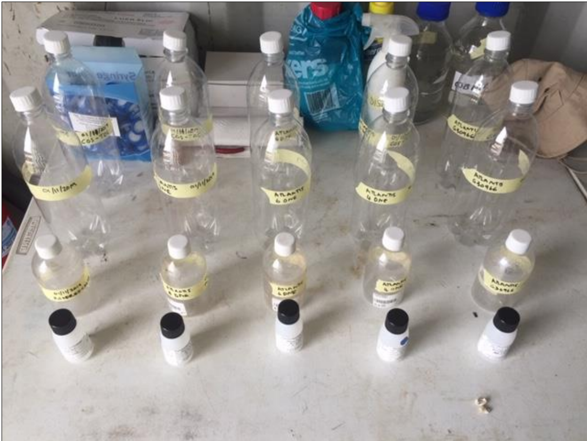
Figure 4.12: Water sampling bottles prepared inside the shipping container at the study site to collect groundwater samples for off-site groundwater chemical analysis
