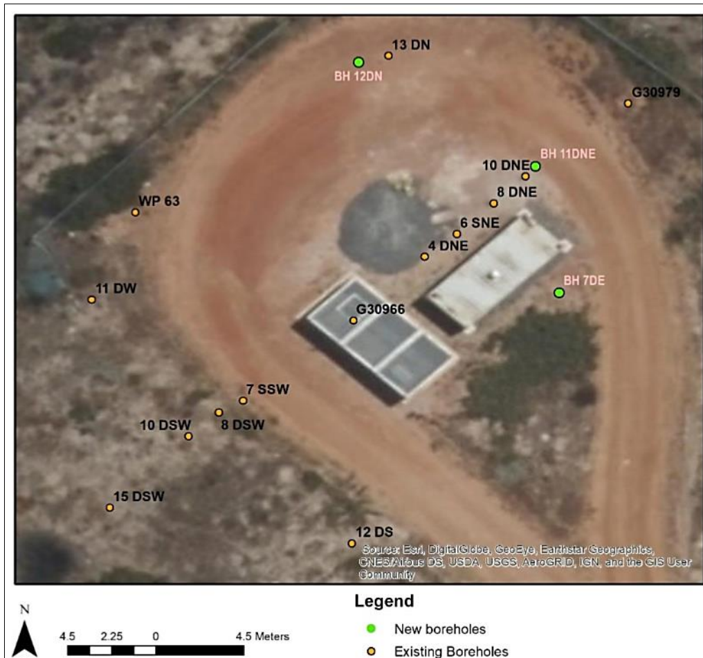
Figure 3.8: Aerial view of the study site in Atlantis representing newly drilled injection boreholes (●), existing monitoring boreholes (●), and the production borehole G30966 (●) (Nhleko et al., 2020). Injection boreholes include 7DE, 11DNE, and 12DN, and existing boreholes include 10DNE, 8DNE, 6SNE, 4DNE, 7SSW, 8DSW, 10DSW, 15DSW, 11DW, WP63, 12DS, 13DN, G3097.
