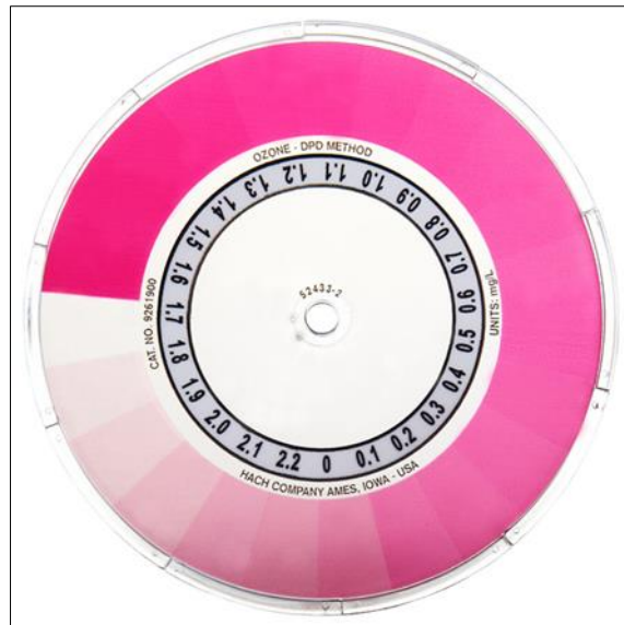
Figure 4.13: HACH Ozone ( O_3 ) Test Kit Model OZ-2 colour wheel measuring O_3 concentration ranges between 0 and 2.2 mg/L in terms of colour intensity.
