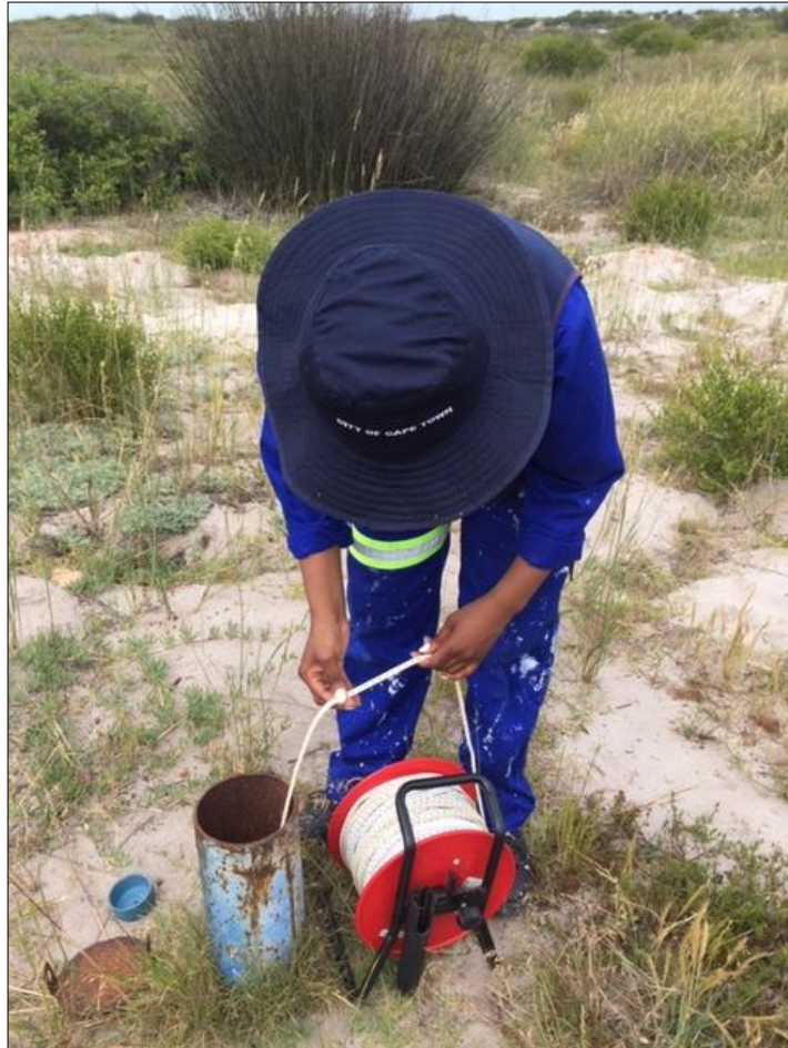
Figure 4.8: Groundwater levels (mbgl) being recorded at 8DSW at the study site in Atlantis using a TLC Water Level Meter.
