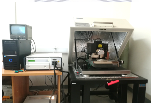
Fig.3.3. Atomic force microscopy instrument used study the topography of Zn-Mo samples.
