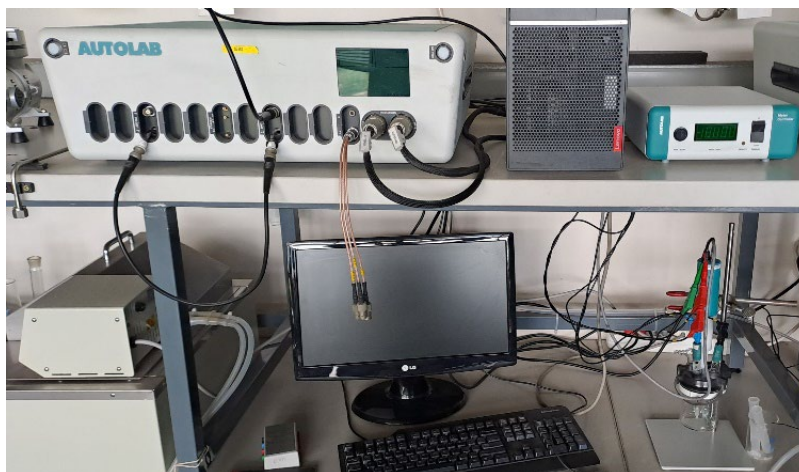
Figure 3.5: The electrochemical measurement set-up.
