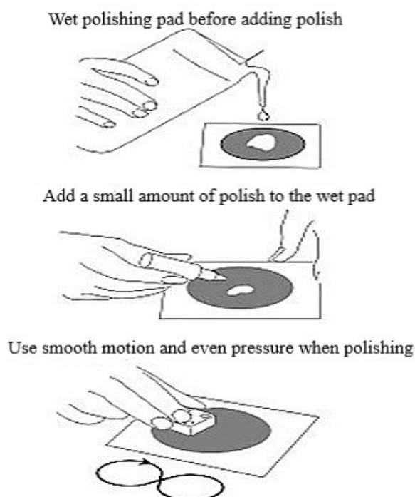
Figure 3.3: Polish and cleaning of the glassy carbon WE.
