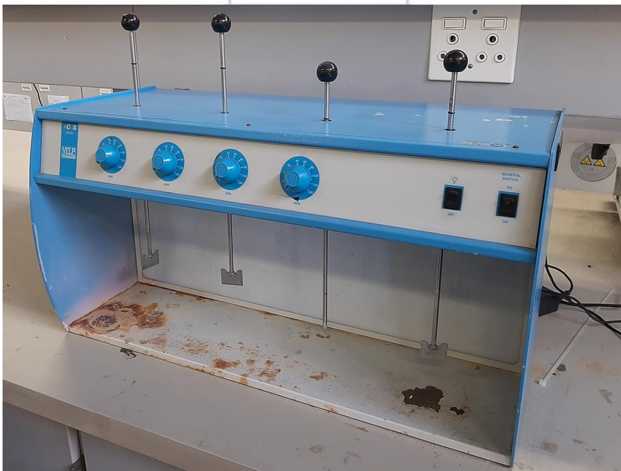
Figure 3.17. Photograph of the VELP Scientific jar test apparatus utilised for the jar tests.
