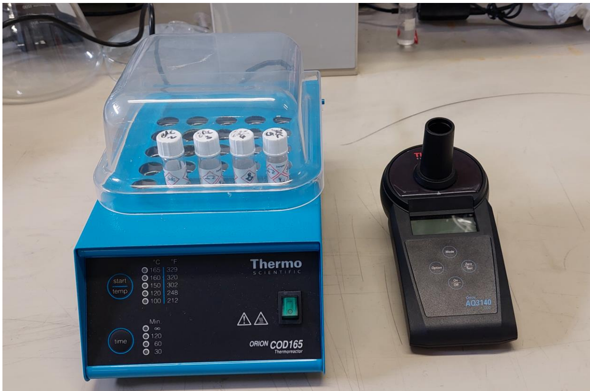
Figure 3.18. COD digester oven and AQ3140 COD colorimeter utilised for the COD measurements.
