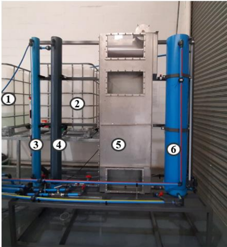
Figure 3.10. Photograph of the hybrid DAF shear unit wastewater system.
