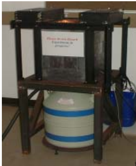
Figure 2.2: The picture shows the lead castle supported by a metallic frame surrounding the HPGe detector.
