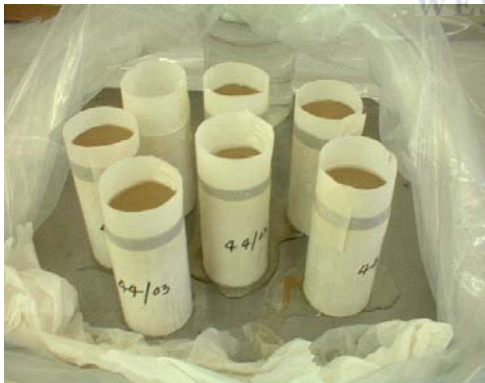
Figure 5.3: Cement blended Solid residue slurry cured in plastic cylinders for strength development testing at Miningtek laboratory.
