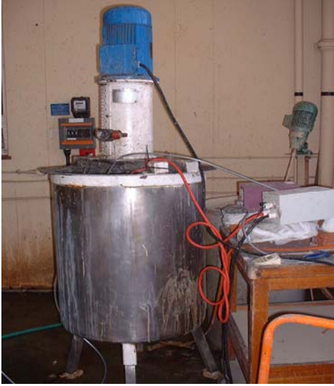
Figure 5.1: The 150 litre capacity agitator used to generate the solid residues used for the drainage experiments.
