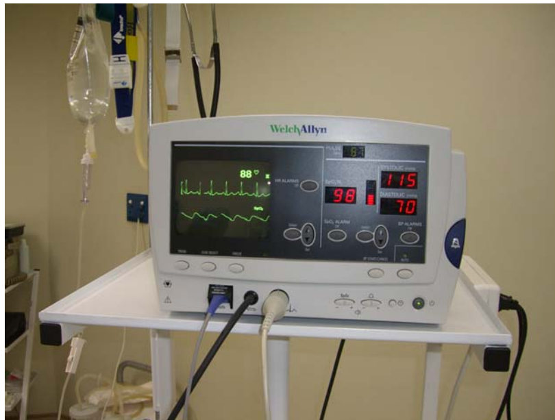
Picture 4 The Welch Allyn monitor used. It measures oxygen saturation levels, ECG, blood pressure and respiration.
