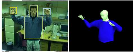
FIGURE 2.6: Micilotta's 3D pose estimation system [56].
