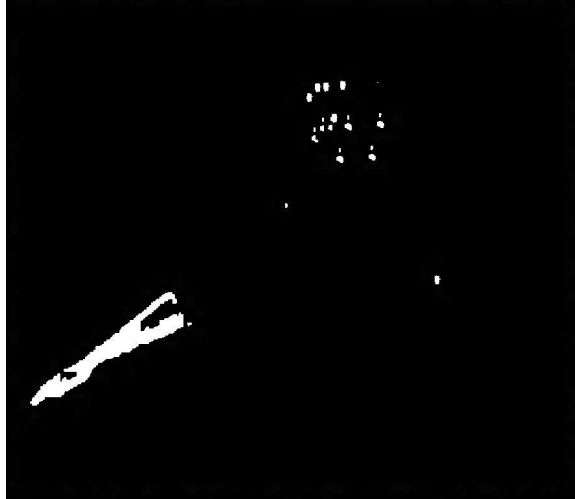
FIGURE 4.7: Result of static background subtraction.
