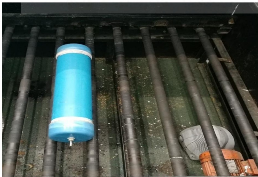
Figure 3.3: High-solids reactor placed on a rig. Heater was placed inside the rig.
