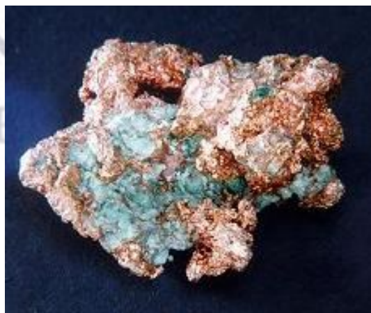
Figure 1.2: A distorted crystal mass picture of copper with typical tarnish green stains. (From the Keweenaw Peninsula of Michigan by Hershel Friedman)
