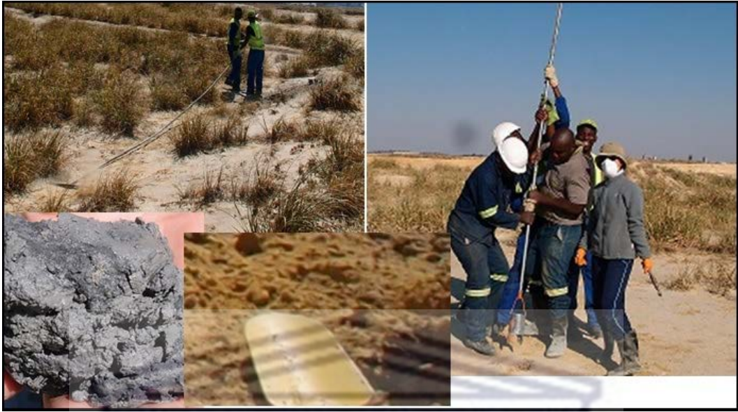
Figure 3.3: Drilling process at Mogale tailings dam
