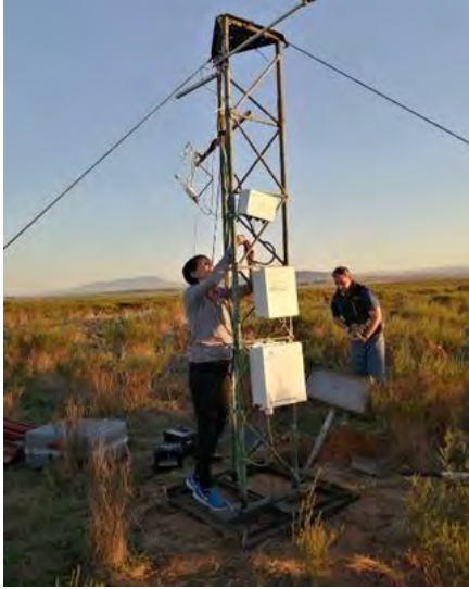
Figure 2.6.: Eddy covariance micrometeorological station in Porterville farm.
