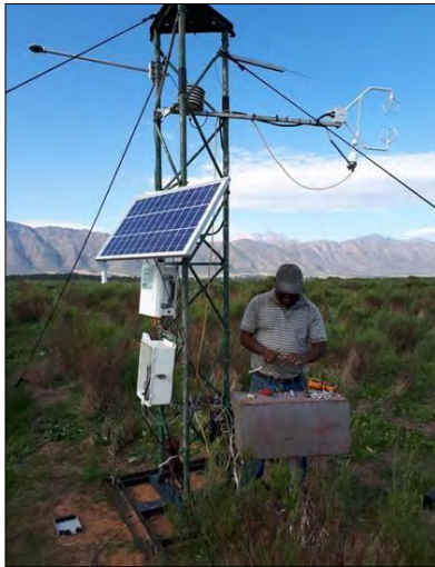
Figure 3.7: Installation of the open path eddy covariance and surface renewal systems over a rooibos crop.
