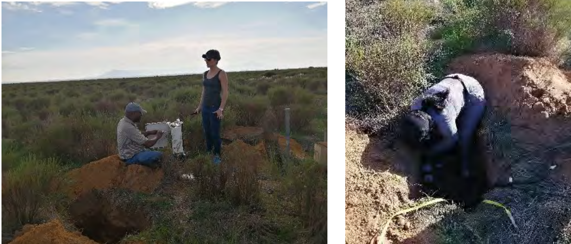
Figure 3.9: Installation of soil moisture sensors to monitor the volumetric soil water content in the root zone of the rooibos crop.
