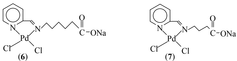
Figure 3.6 \omega -carboxylato ligand complexes in which \text{PdCl}_2(\text{CH}_3\text{CN})_2 was used as palladium source
