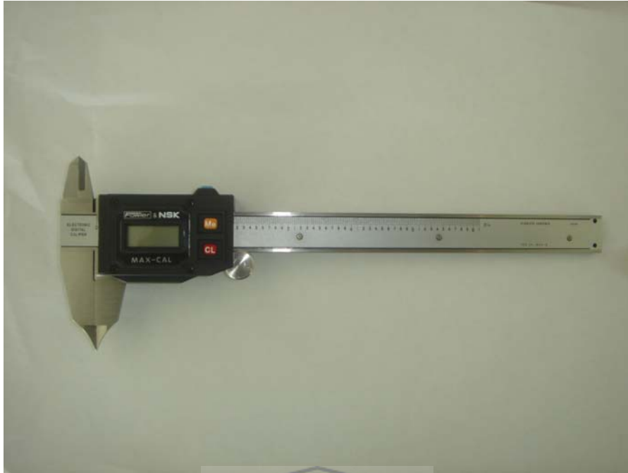
Figure 1 MAX-CAL electronic digital caliper. MAX-Series electronic digital Caliper with a resolution of 0,01mm, Fowler & NSK, made in Japan.
