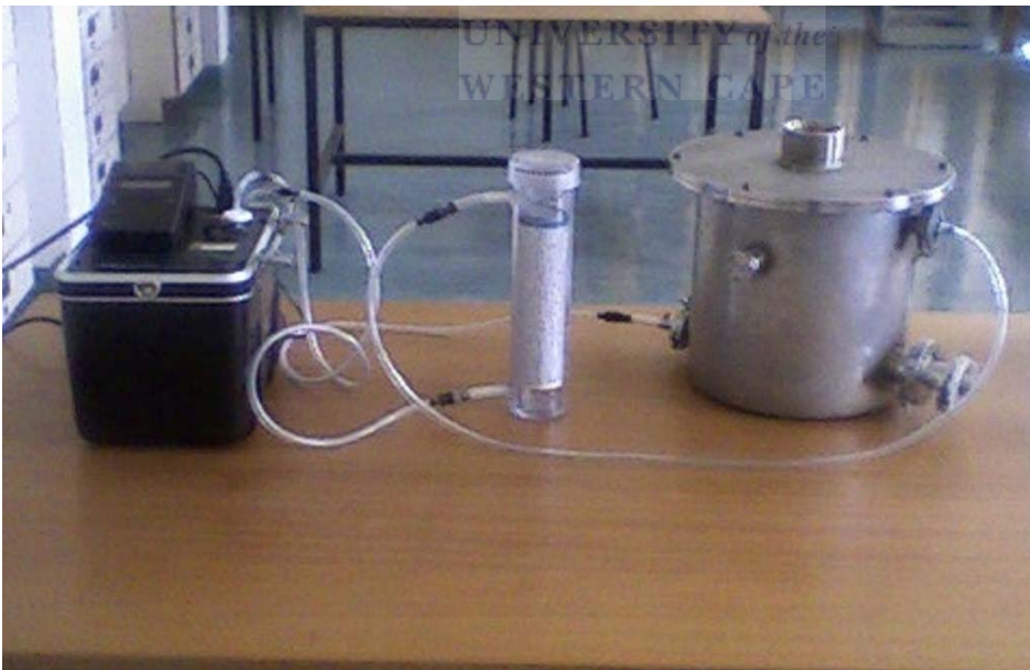
Figure 4.9 (a): The radon experiment before the introduction of the ice
