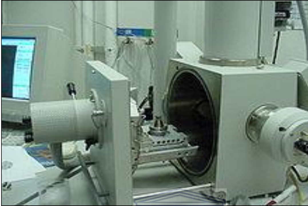
Figure 4.3: Scanning Electron Microscopy Machine/EDS (Physics Department, UWC)
