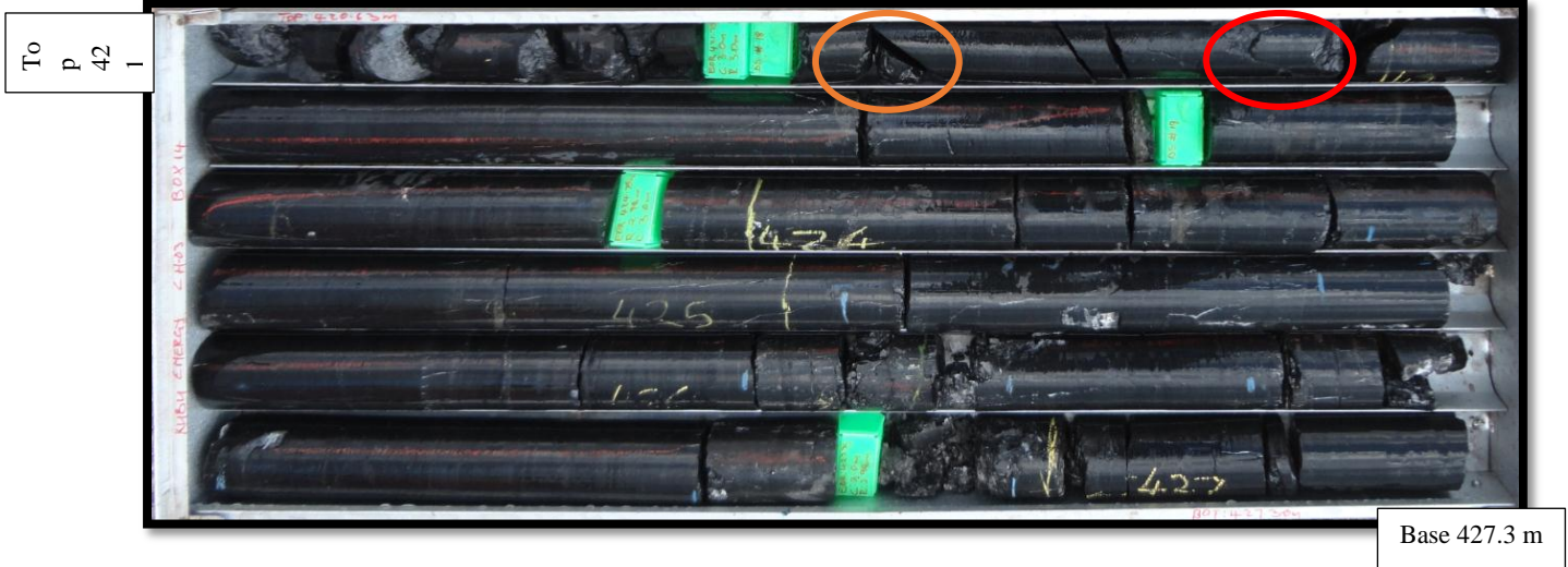
Figure 32 Coal interval Z1 as observed on well C3 with high angled fractures orange circle and low angled fractures red circle at depths of 421.55-422.82m. The sub-horizontal cracks are stress release structures.
