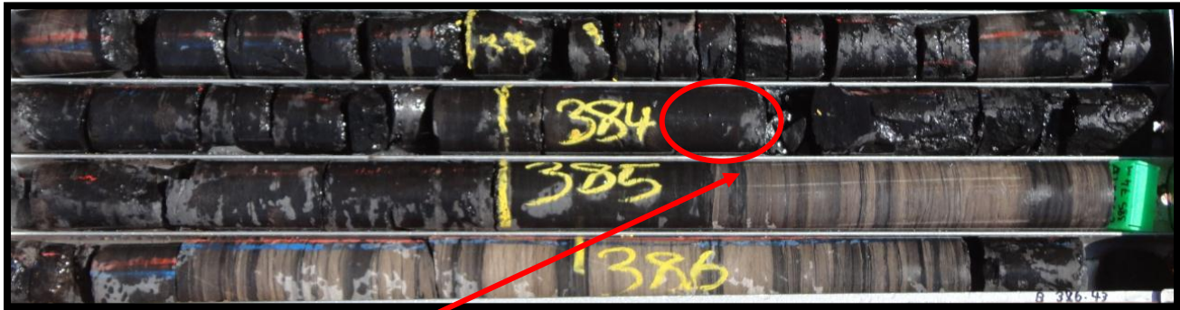
Figure 31 Carbonaceous mudstones with coal stringers from well C2. Note also the distinct bedding lamination along the red arrow position.
