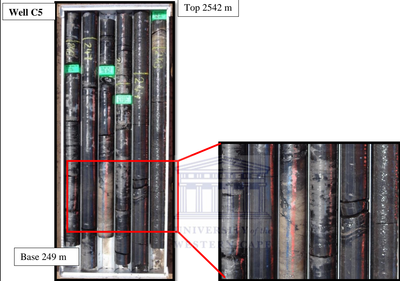
Figure 24 Normal light core image taken when un-slabbled core was wet. UMH 1 core from well C1. Abundant calcite micro-cleats in brittle core zones.
