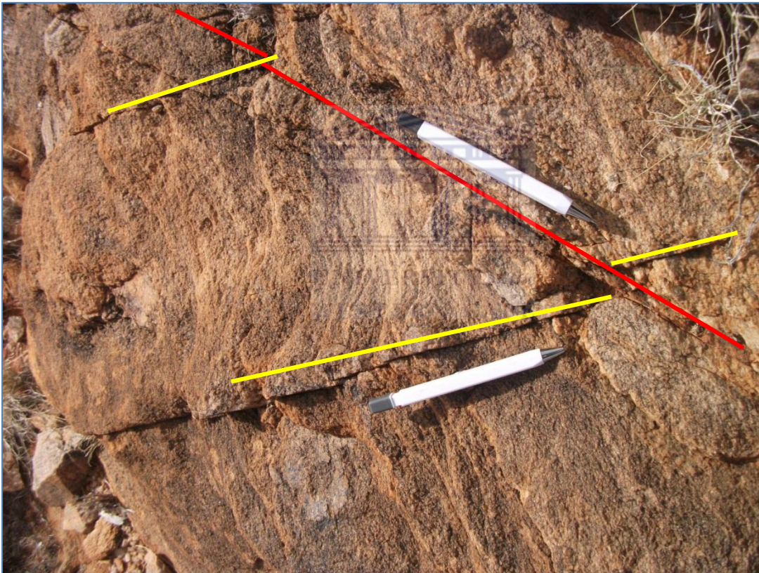
Figure 7.17 Quartzite showing conjugate joints. At the top left corner of the red joint has been displaced by the yellow one which means that red formed first. At the bottom right corner the yellow is displaced by red which means that red formed later.
