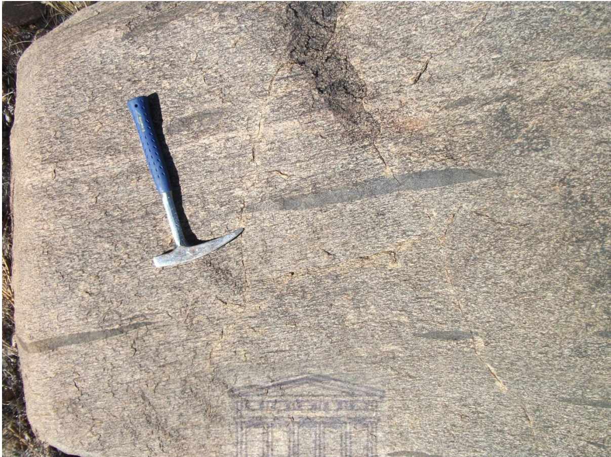
Figure 8.3 Granitoid with lenticular mafic xenoliths parallel to direction of foliation
