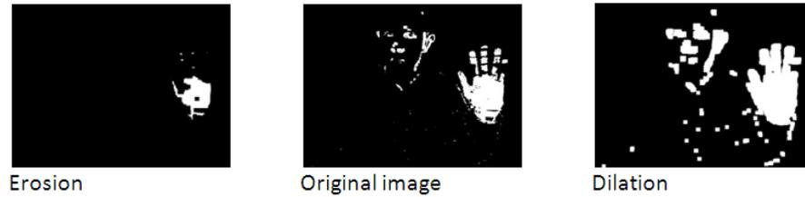
FIGURE 4.3: Dilation and erosion.
