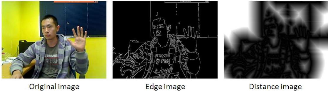
FIGURE 3.12: An edge image converted to a distance image using the distance transform algorithm.
