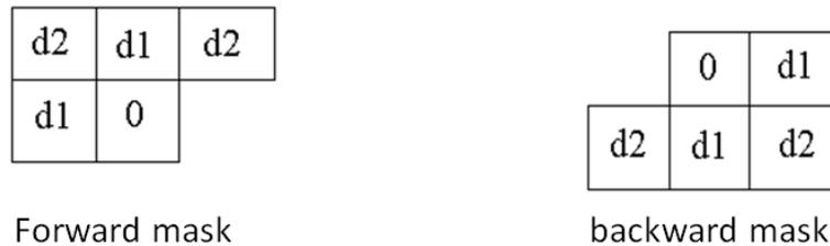
FIGURE 3.13: The  $3 \times 3$  mask with value ( $d1=4, d2=3$ ) distance transform.
