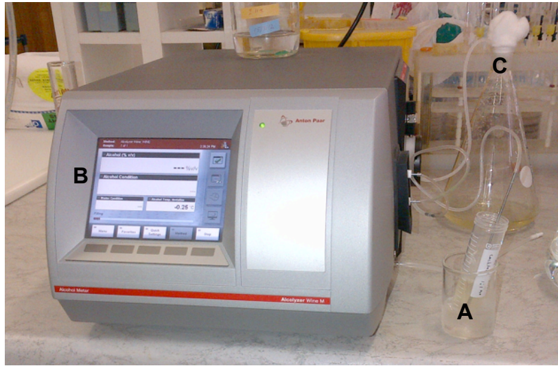
Figure 2.1: This figure demonstrates the sequential events of alcohol analysis by the alcolyzer wine M. (A) Is the inlet where the sample is suctioned and flows through the duct for alcohol detection. (B) The monitor that displays the amount of alcohol in the solution after detection. (C) Is the outlet; post analysis the sample is discarded as waste through this channel.
