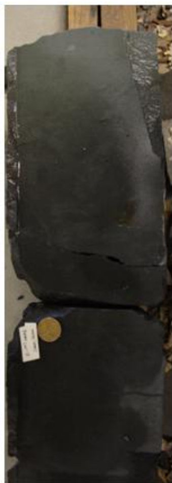
Plate 12: Showing highly bioturbated, muddy-siltstone at 2600.20 m. Coin diameter: 1.7cm
