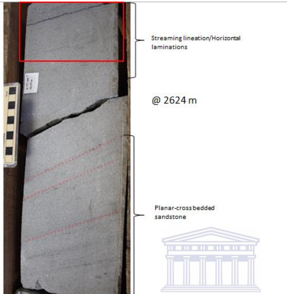
Plate 3: Showing sandstone with planar-cross beds and streaming lineation and/or horizontal laminations at 2624 m.
