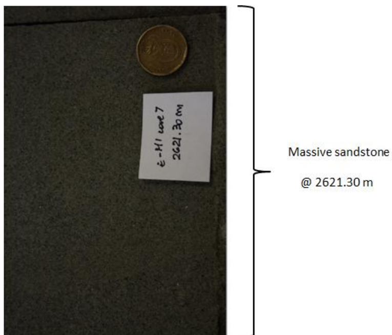
Plate 4: Facies 5, massive sandstone of a tidal bar, taken from 2621.30 m. Coin diameter: 1.7cm
