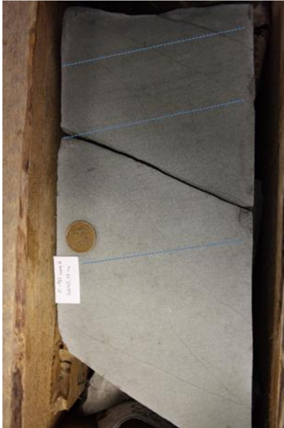
Plate 7: Showing faint lamination on fine silty sandstone at 2610.11 m. Coin diameter: 1.7cm
