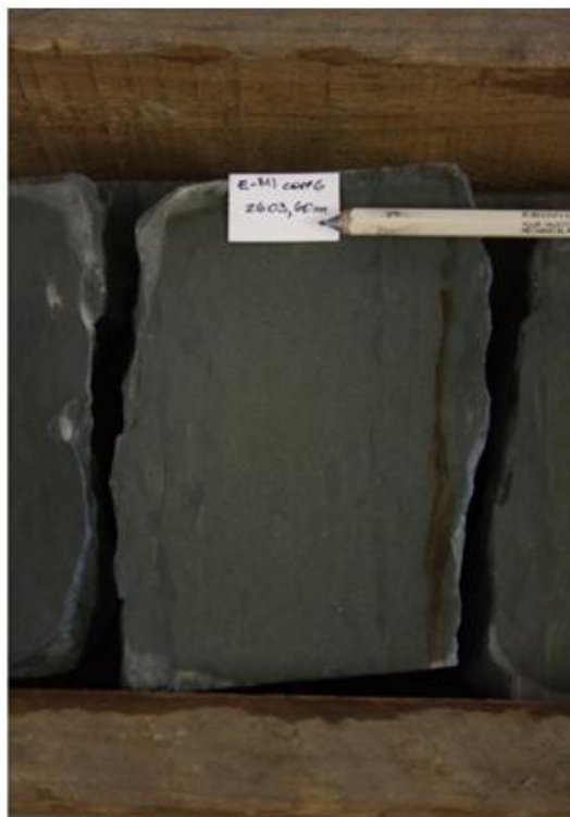
Plate 10: Showing bioturbated siltstone from the transitional zone at 2603.60 m. Pencil length: 15cm
