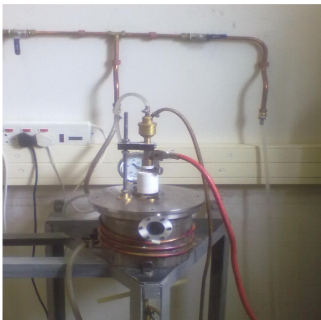
Figure II-1: Arc-melting furnace chamber at the University of the Western Cape (Physics Department), similar to that utilized at Wits University.
