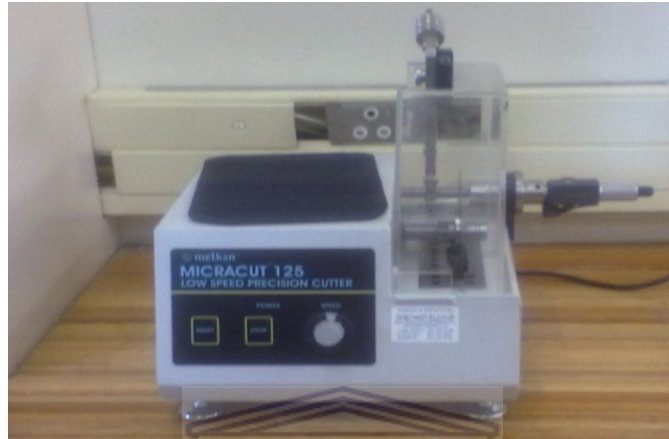
Figure II-3: Micracut 125 low speed cutter at the University of the Western Cape (Physics Department).
