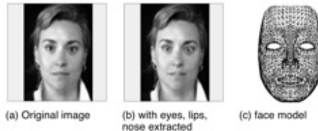
Figure 4.9: Feature tracking to fit a 3D model on to a face (41)
