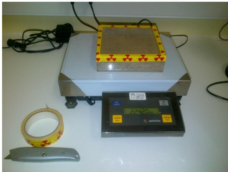
Figure 3.13: A photograph of the soil sample in a new measuring geometry on a mass scale sealed using tape.
