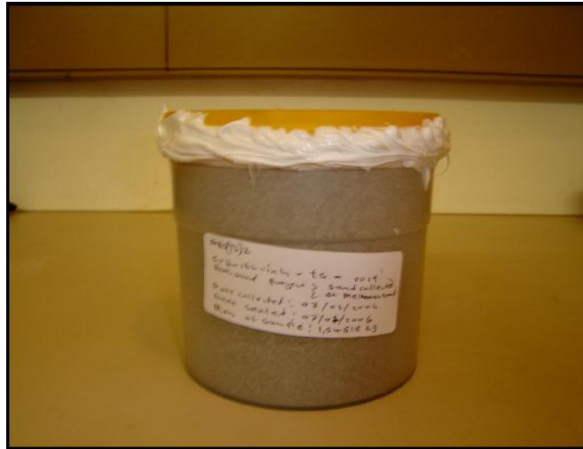
Figure 3.11: A typical photograph of a sealed Marinelli beaker with the soil sample inside.
