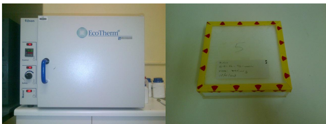
Figure 3.14: Photographs showing the ERL EcoTherm oven (left-side) used in this study to dry the samples and the KCl sample in a container (right-side).
