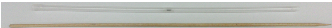
Figure 3.9: Picture showing sample mounted in the straw for the magnetization and magnetic susceptibility measurements on MPMS.
