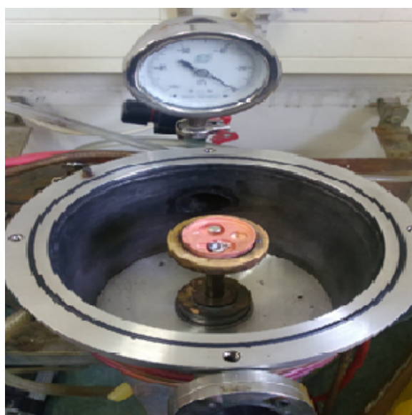
Figure 3.1: The figure showing the arc-furnace chamber, with the titanium and the starting elements placed in the appropriate copper crucible.
